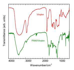
Figure 4. Fourier transform infrared (FT-IR) spectroscopy result of vinylon and PANI/vinylon composite
