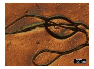
**Figure 2.** A circular polarized interference optical microscopy (C-DIM) image of vinylon.
