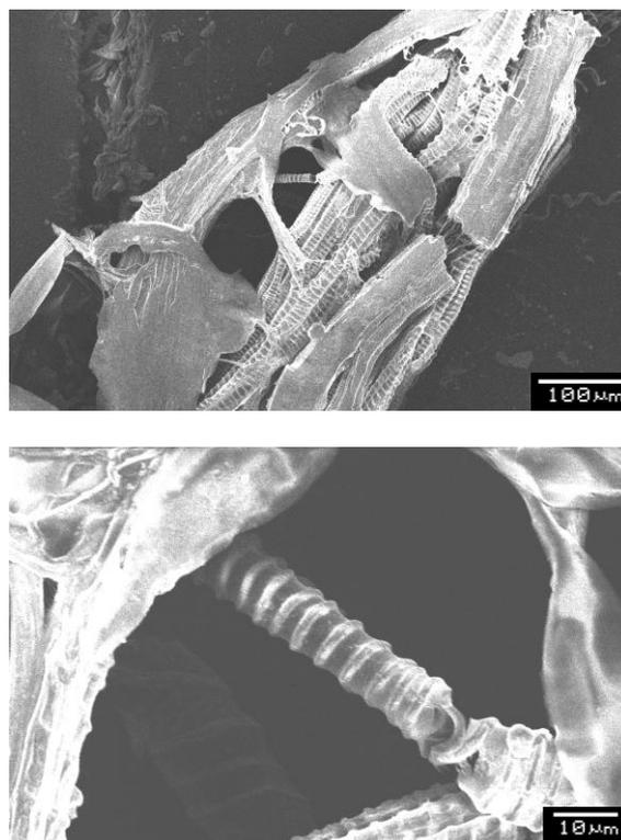
**Figure 3.** SEM images of helical vessels dyed by poly1. a) Entire image of the polymerization-dyeing helical vessels. Magnification image of the helical vessel coated by the azo-polymer (poly1). Maintaining after polymerization-dyeing can be confirmed.
