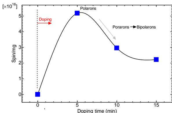
**Figure 5.** In-situ electron spin resonance (ESR) spectroscopy measurements of the polymer with iodine vapor doping.
