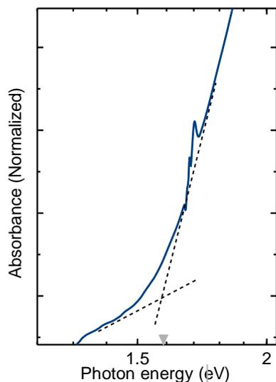
**Figure 4.** Band-gap energy of poly(DN-ITN).
