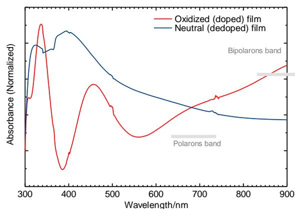
**Figure 3.** UV-vis absorption spectra of poly(DN-ITN).
